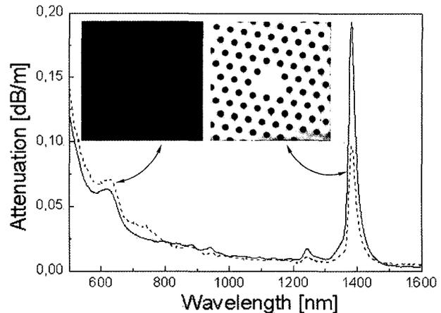
Fig. 4. (a) Loss curves for the two large mode-area fiber designs shown in the insets. The fiber with three holes removed (right) has a mode field diameter of  $12 \mu\text{m}$ , whereas the fiber with one hole removed (left) has a mode field diameter of  $10.5 \mu\text{m}$ .
