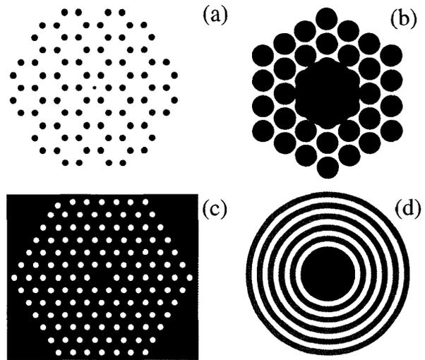
Fig. 6. Schematic pictures of various photonic bandgap (PBG) fiber designs. Lighter color indicates higher refractive index. (a) Honeycomb PBG fiber with central hole defect. (b) Airguiding PBG fiber. (c) PBG fiber with a triangular array of high-index rods, formed e.g. by liquid-filling of the holes in a standard index-guiding PCF. (d) Omniguide PBG fiber.
