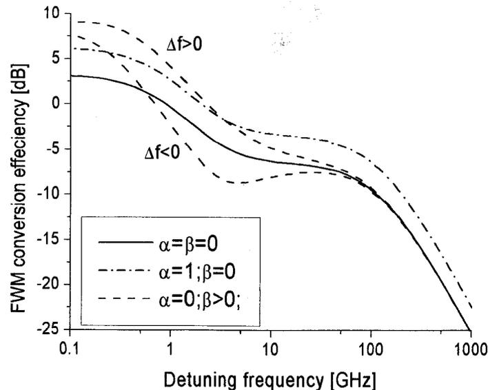
Fig. 3: Conversion efficiency for non-zero linewidth enhancement factors  $\alpha$  and  $\beta$ .
