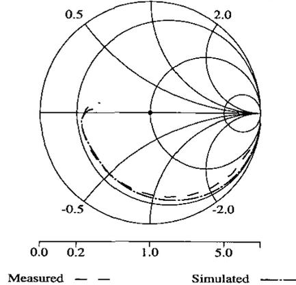
**Figure 7.** Simulated and measured reflection coefficient ( $s_{11}$ ) of the MEMS tunable capacitor from 45 MHz to 10 GHz. Simulations are run using the equivalent circuit given in Figure 2, with measured values of  $C_I$ ,  $R_s$ ,  $C_{P1}$  and  $C_{P2}$ , and estimated values of  $R_{sub}$  and  $L_s$ .
