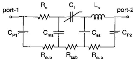
Figure 2. Equivalent circuit of the MEMS varactor.
