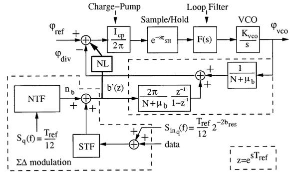
Fig. 6. Complete linearized sample-hold  $\Sigma\Delta$  fractional- $N$  PLL.
