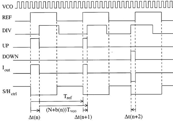
Fig. 5. PLL waveforms.
