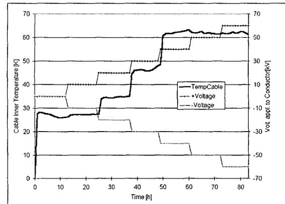
**Fig. 3:** Variation of Voltage or Temperature with time
