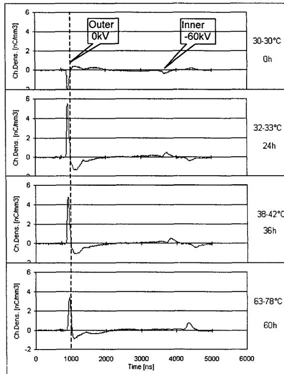
**Fig.5:** Space charge distribution in 24kV, XLPE cable with negative polarity: -15kV/mm, DC for 60hours with the temperature between conductor and outer semicon increasing from 30-30 to 63-78°C. Sample 3
