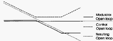
Figure 15. Combining inner and outer loop functions
