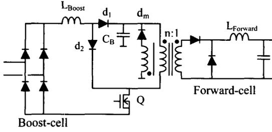
Figure 2. Single-Stage Power Supply Using Boost-Forward Topology.
