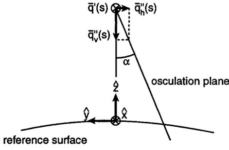
Fig. 1: Satellite orbit  $\bar{q}(s)$  with an acceleration (curvature) in both the vertical direction,  $\bar{q}''_v(s)$ , and the horizontal direction,  $\bar{q}''_h(s)$ . The osculation plane of the orbit has an angle,  $\alpha$ , with the vertical.
