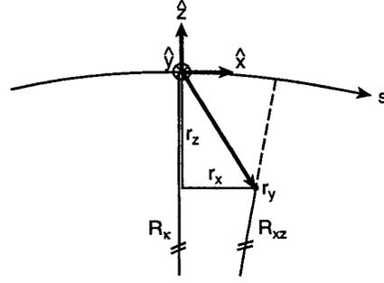
Fig. 2: Satellite track with a radius of curvature,  $R_\kappa$ , approximated by a circle in the osculation plane  $(x, z)$ , where  $\hat{x} = \hat{t}_0$ ,  $\hat{y} = \hat{b}_0$ , and  $\hat{z} = -\hat{n}_0$ . A target is assumed at a known position  $(r_x, r_y, r_z)$ .
