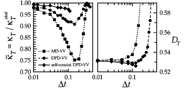
FIG. 2. Left: Dimensionless isothermal compressibility  $\tilde{\kappa}_T$  vs  $\Delta t$  for the integrators shown in the legend. Right: Tracer diffusion coefficient  $D_T$  vs  $\Delta t$  for the same integrators.
