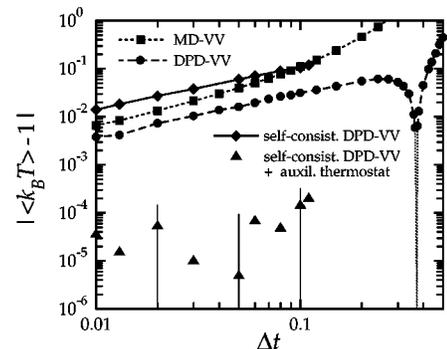
FIG. 3. Double-logarithmic plot of the modulus of the deviation of  $\langle k_B T \rangle$  from the desired temperature  $k_B T^* \equiv 1$  vs  $\Delta t$ . For self-consistent DPD-VV with auxiliary thermostat,  $1\sigma$  error bars are shown for some of the data points.
