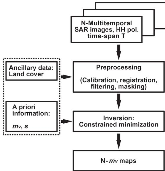
Fig. 1. Flowchart of the soil moisture retrieval algorithm.
