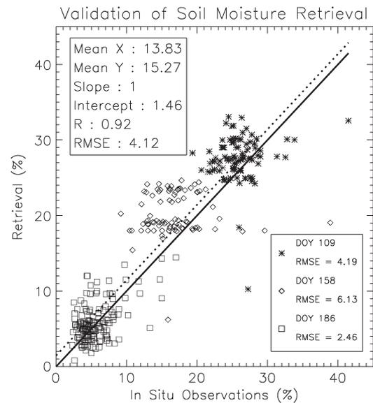
Fig. 3. Validation of the retrieved soil moisture values using the *in situ* observations. The solid line is the 1:1 line, the dotted line the regression line. The different symbols indicate different dates as explained in the bottom right-hand side legend.
