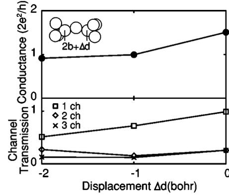
FIG. 2. Conductance (top) and channel transmissions (bottom) at the Fermi energy for three-Al-atom wires as a function of displacement of electrode spacing,  $\Delta d$  (fixed atom-atom bond length). For the atom bases contacting the jellium electrode, a triangular shape is used. (1 bohr=0.529 Å).
