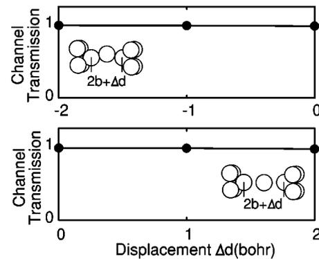
FIG. 10. First channel transmissions (conductance in unit of  $G_0$ ) for three-atom-long Na wires with rectangular atom bases contacting the jellium electrodes. The top and the bottom panels show the transmissions as a function of displacement of electrode spacing,  $\Delta d$ .
