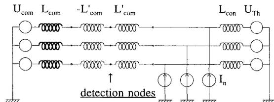
Fig. 8. Converter AC side equivalent diagram with detection circuit.
