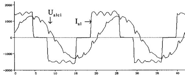
Fig. 9. Measured voltage and current. Time (ms)
