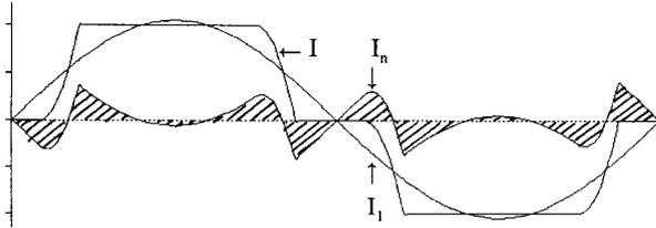
Fig. 7. Converter line, harmonic, and fundamental frequency currents.
