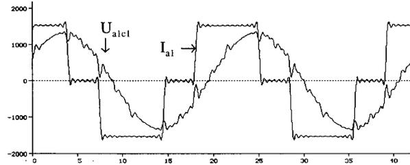
Fig. 11. Simulated voltage and current with harmonics up to 37<sup>th</sup>. Time (ms)
