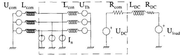
Fig. 6. Converter equivalent diagram.
