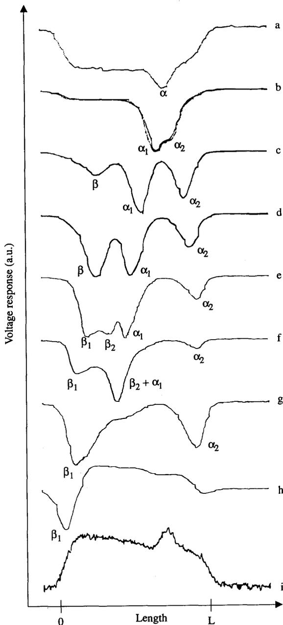
Fig. 3. Line-scans showing the voltage response when biased at the points a-i in Fig. 2. The response voltage is shown as function of the beam position. The line-scans are shown off-set for clarity. Due to slight changes in the amplification, the voltage response for the different biaspoints can only be compared qualitatively. The total scanning range is  $300 \mu\text{m}$ .
