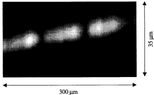
Fig. 1. Quasiparticle distribution in a part of a  $5 \mu\text{m}$  wide inhomogeneous long Josephson tunnel junction. The inhomogeneities are spaced  $100 \mu\text{m}$  apart and are  $5 \mu\text{m}$  wide. Dark regions correspond to low voltage response signal, white to maximum signal. The picture shows a sample area of  $300 \times 35 \mu\text{m}^2$ .
