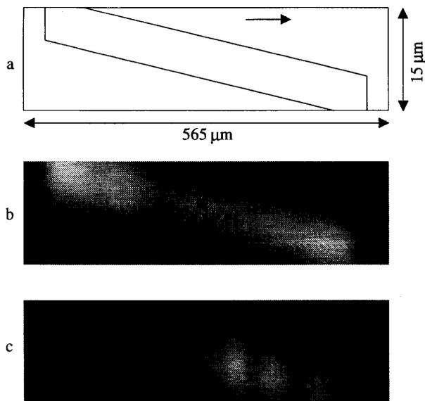
Fig. 4. a)–Sketch of the  $500 \times 5 \mu\text{m}^2$  large junction. The arrow indicates the scan direction in b) and c). b)–Voltage response from the junction when biased in the subgap regime at  $V=2.4 \text{ mV}$ . c)–Voltage response with the junction biased at  $V=700 \mu\text{m}$  with an applied magnetic field.
