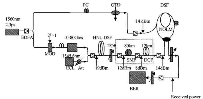
Fig. 1. Experimental setup for 80 Gb/s wavelength conversion and transmission. EFRL: erbium fiber ring laser, MOD: LiNbO<sub>3</sub> modulator, MUX: 10–80 Gb/s multiplexer, NOLM: nonlinear optical loop mirror, SMF: single mode fiber, DCF: dispersion compensating fiber, TOF: tunable optical filter, ECL: external-cavity laser, OTD: optical time delay, Att: attenuator.
