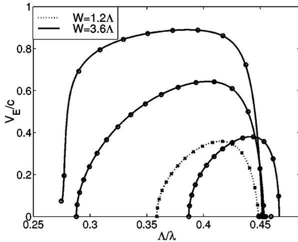
FIG. 8. Energy propagation velocity for guided modes in the two-dimensional photonic crystal waveguide for two choices of the waveguide width  $W$ . The smooth curves were obtained directly from the dispersion relations by calculating  $d\omega/dk_x$ , whereas the discrete points were obtained using Eq. (4).
