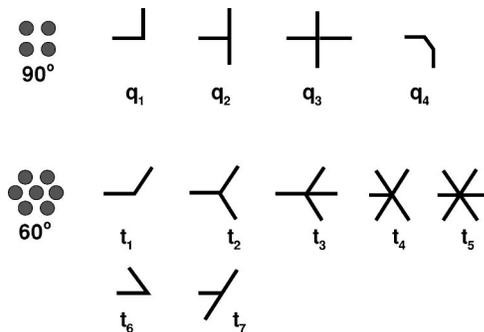
FIG. 11. Quadratic (90° symmetry) and triangular (60° symmetry) lattice crystals with some of the most obvious configurations of waveguide connections (branching points) for the redistribution of energy.
