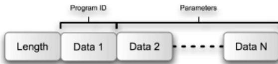
Fig. 13. Transmission package structure.
