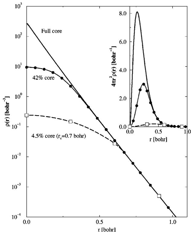
FIG. 4. The full all-electron core density and the partial core densities used in the PP-4.5%-O-core and PP-42%-O-core oxygen pseudopotentials. In the inset the spherical Jacobian factor  $4\pi r^2$  has been included. A denser sampling (black circles) is required for PP-42%-O core compared to PP-4.5%-O core (open squares).
