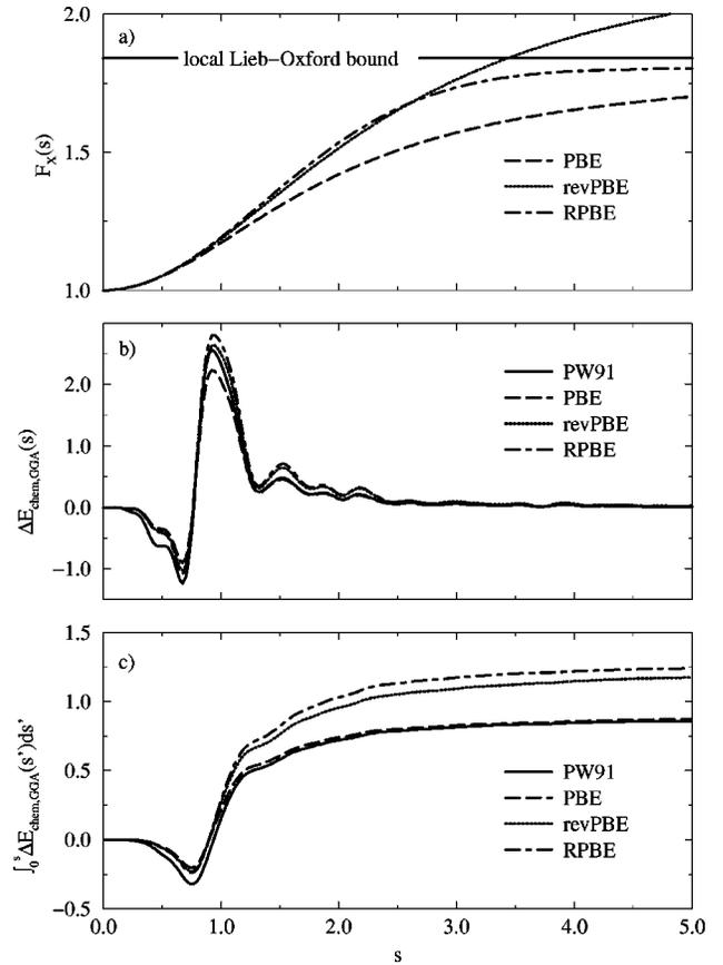
FIG. 3. (a) The exchange enhancement factor for the different GGA functionals as a function of the reduced density gradient,  $s$ . (b) The distribution of nonlocal exchange-correlation energy contributions,  $\Delta E_{chem,GGA}(s)$ , to the chemisorption energy of CO on Pd(100). (c) The integrated distribution of nonlocal exchange-correlation energy contributions to the chemisorption energy of CO on Pd(100).
