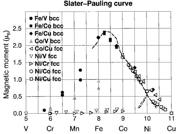
FIG. 2. The averaged interface moment  $m_{AB}^{IF}(\tilde{N})$ , Eq. (1), as a function of valence charge  $\tilde{N}$  for the different magnetic interfaces (Slater-Pauling curve). The dashed lines show the experimental moments for FeV, FeCo, CoNi, NiCu, and NiCr alloys. The dot-dashed line shows the moment for the NiV alloy.
