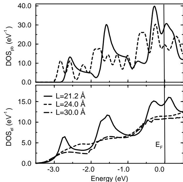
FIG. 4. Upper: Density of states (DOS) inside the unit cell in the self-consistent calculation for  $L = 21.2 \text{ \AA}$  (solid line) and  $L = 24.0 \text{ \AA}$  (dotted line). For clarity we do not show the very peaked DOS for  $L = 30.0 \text{ \AA}$ . Lower: Local DOS (integrated over the part of the wire in between the electrodes) for the nanowire coupled to the electrodes. The DOS is seen to be quite smooth after the first restructuring.
