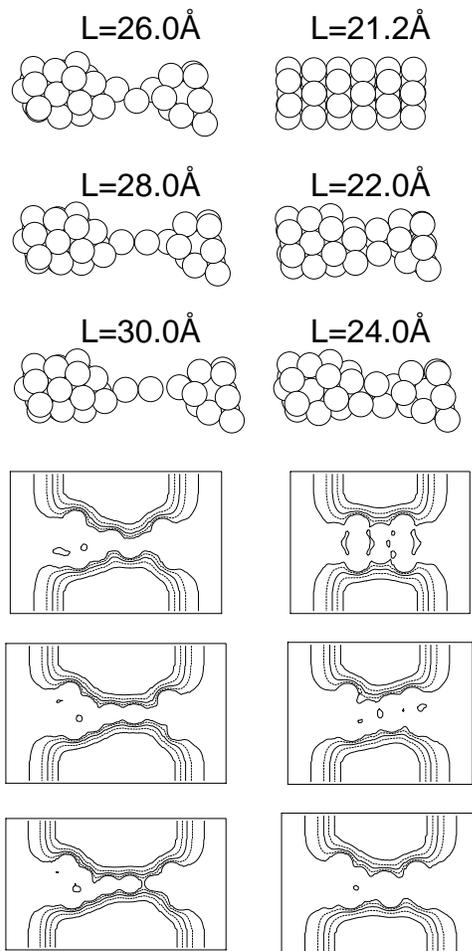
FIG. 1. Calculated atomic structures for different heights,  $L$ , of the unit cell. Periodic boundary conditions are applied in the calculation. Below, the corresponding cross-sectional contours ( $E - E_F = -3, -2, \dots, +1$  eV) of the potentials constructed for the transmission calculation.
