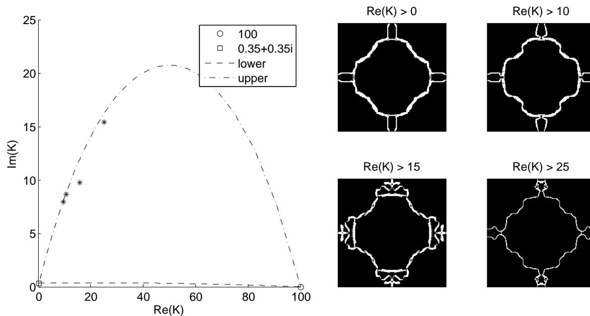
Figure 1: The figure shows the optimized material structures that approach the upper bound. The structures are made from two isotropic materials with equal Poisson's ratio of 0.3. One constituent (black) is a relatively stiff elastic material while the other (white) is a more compliant viscoelastic material having a bulk modulus of  $K_1 = 100$  and  $K_2 = 0.35 + 0.35i$
