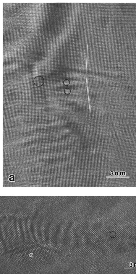
FIG. 2. HRTEM images of bcc grains in a  $\text{Fe}_{50}\text{Cu}_{50}$  sample after 30 h of MA. (a) The white-edged black lines indicate a deviation of about  $5^\circ$  between the lower and upper part of the grain. The circles indicate some edge dislocations with  $\mathbf{b} = 1/2[110]$ . (b) An elongated needlelike bcc grain. The circle and asterisk indicate a dislocation and a lattice distortion region, respectively.
