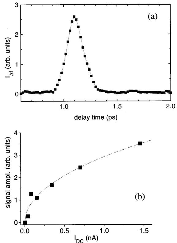
FIG. 3. (a) Delay time dependent tunneling current measured at  $V_h = 48 \text{ mV}$ ,  $I_{DC} = 0.7 \text{ nA}$  with the tip under the probe beam. (b) Amplitude dependence on  $I_{DC}$ . The data are compared to a fit function  $y = a x^b$  with  $b = 0.49$ .
