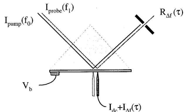
FIG. 1. Experimental setup for time resolved reflectivity and tunneling current measurements. Pump and probe beams are modulated at  $f_0$  and  $f_1$ , respectively, with a difference frequency of  $\Delta f$ . The change in reflectivity (tip position indicated by dotted outline) and the change in the tunneling current (full tip outline) are measured at  $\Delta f$ . The laser wavelength is 840 nm and the pulse width 100 fs.
