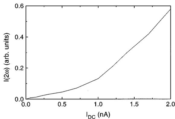
FIG. 4. Second harmonic tunneling current contribution,  $I(2\omega)$ , for a bias modulation at  $\omega=2.4$  kHz.  $I_{DC}$  is set average tunneling current, the bias voltage is  $V_b=48$  mV, and the voltage modulation amplitude is  $V(\omega)=10$  mV.
