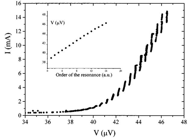
FIG. 5. Example of fine structures on the profile of the zero-field singularity for sample B measured at  $T = 1.8 \text{ K}$ . The inset demonstrates that the fine structures are almost equally spaced.
