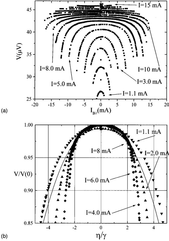
FIG. 3. (a) Magnetic tuning of the single fluxon voltage at different bias points along the ZFS1 for sample B at  $T=4.2$  K. (b) Low-bias data of (a) in normalized units; for each bias current  $V(0)$  is the step voltage in zero magnetic field. The full line is the analytic expression (4).
