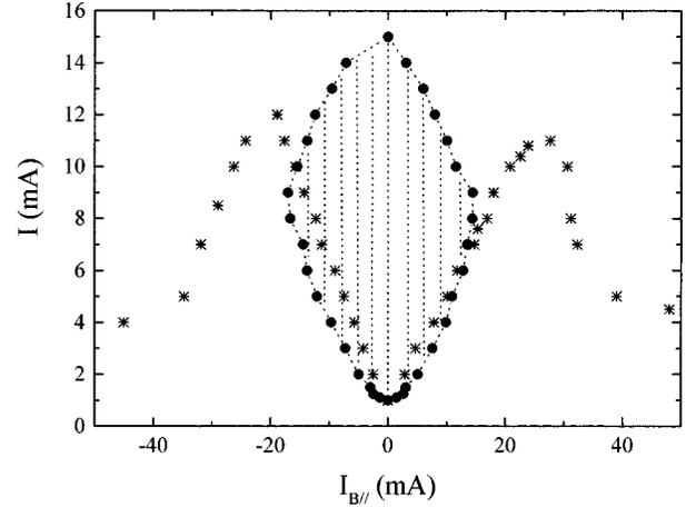
FIG. 2. Magnetic pattern of the critical current (stars) for sample B with one trapped fluxon in a current-parallel magnetic field  $B_{\parallel}$  proportional to the current  $I_{B_{\parallel}}$  flowing in the coil. The hatched area delimited by the dots shows the range of existence of the traveling fluxon mode in the  $I$ - $B_{\parallel}$  plane.
