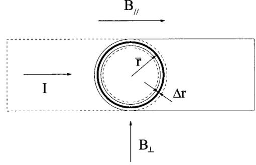
FIG. 1. Schematic of our annular Nb/Al-AIO<sub>x</sub>/Nb junctions. The base electrode (dashed line) is slightly larger than the wiring film (full line). The tunnel barrier is shown by the black area.
