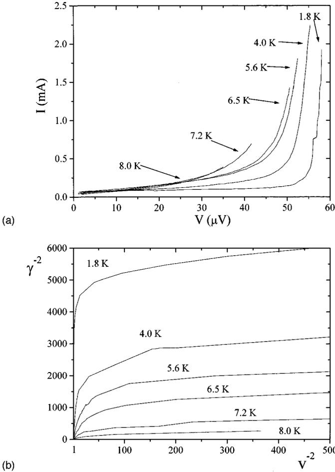
FIG. 4. (a) ZFS1 profile for sample A at different temperatures; (b) the same data of (a) plotted as  $\gamma^{-2}$  versus  $v^{-2}$ .  $\gamma$  is the distributed bias current  $I$  normalized to  $I_0(T)$  and  $v$  is the junction voltage  $V$  divided by the temperature-dependent asymptotic voltage.
