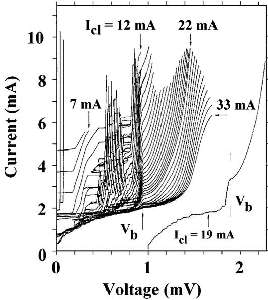
FIG. 2.  $I$ - $V$  characteristics of a test FFO recorded at different applied magnetic fields supplied by the control line current  $I_{cl}$ . The increment  $\Delta I_{cl}$  is 0.5 mA for  $7 \text{ mA} < I_{cl} < 22 \text{ mA}$ , while  $\Delta I_{cl} = 1 \text{ mA}$  for  $22 \text{ mA} < I_{cl} < 33 \text{ mA}$ . The inset (shifted by 1 mV) shows the definition of the “boundary” voltage  $V_b$  for one of the  $I$ - $V$  characteristics, recorded at  $I_{cl} = 19 \text{ mA}$ .
