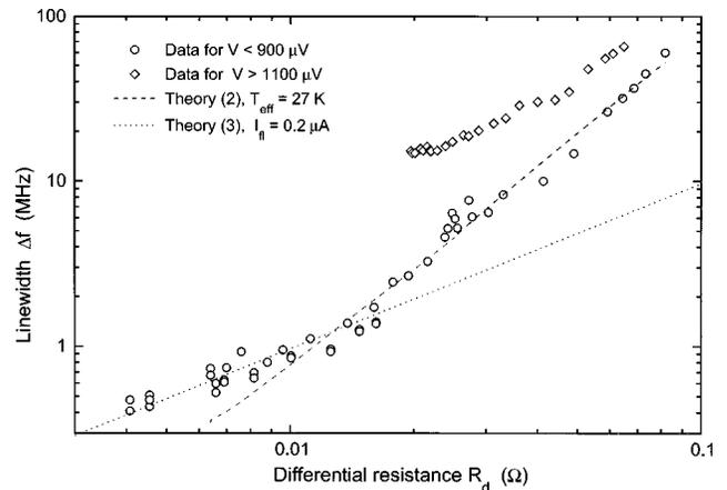
FIG. 6. Dependence of the linewidth  $\Delta f$  on the differential resistance  $R_d$ . Data are recorded at  $V < 900$   $\mu$ V (circles) and  $V > 1100$   $\mu$ V (diamonds). Theoretical dependence [Eq. (2)] for the lumped (short) tunnel junction with  $T_{\text{eff}} = 27$  K is shown by the dashed line; the dependence [Eq. (3)] for a low-frequency noise current  $I_{\text{lf}} = 0.2$   $\mu$ A is presented by the dotted line.
