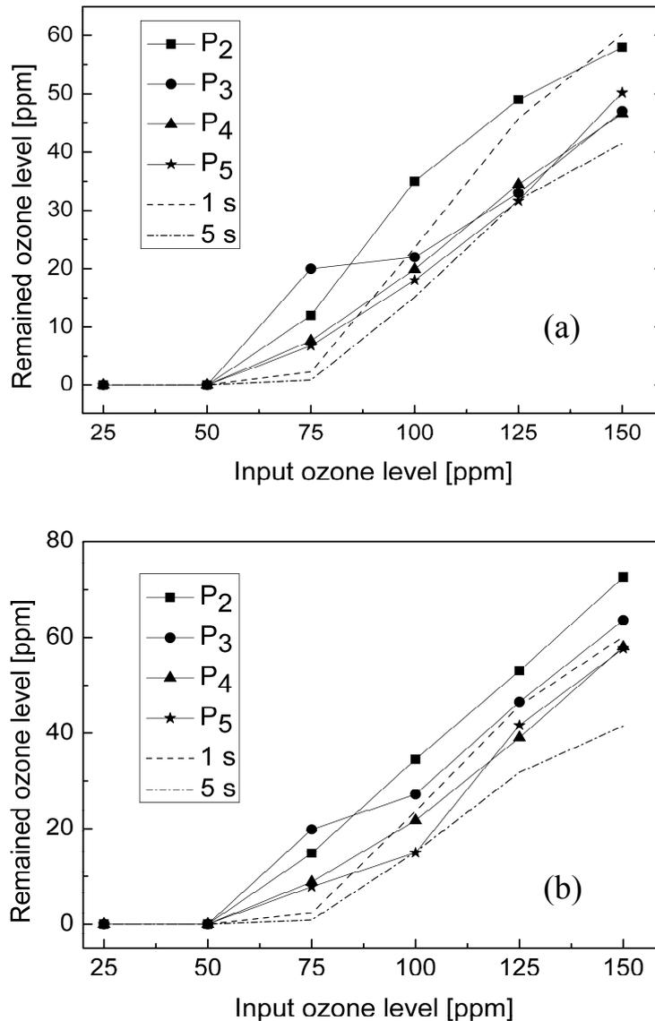
Fig. 6 Ozone concentrations at ports  $P_2$ - $P_5$  as a function of ozone input level measured by (a) FTIR and (b) UV absorption. Dashed lines show the simulated ozone concentration for a residence time of 1 and 5 sec, respectively where,  $NO=80$  ppm and  $T=60$  °C.
