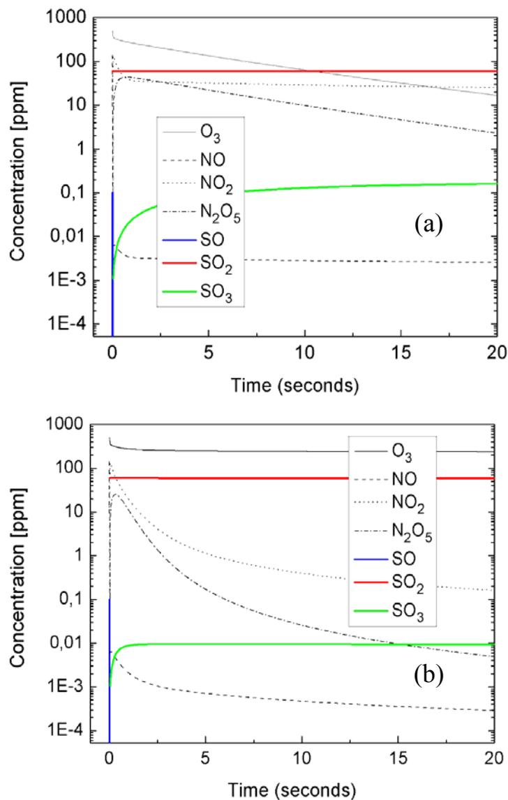
Fig. 10 Calculated evolutions of O<sub>3</sub>, NO, NO<sub>2</sub>, N<sub>2</sub>O<sub>5</sub>, SO, SO<sub>2</sub> and SO<sub>3</sub> concentrations in the reactor during 20 seconds after ozone injection, (a) no water and (b) including 10 μm water droplets.
