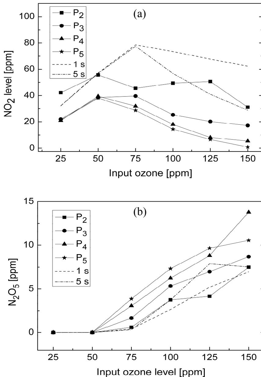
Fig. 8  $\text{NO}_2$  (a) and  $\text{N}_2\text{O}_5$  (b) with simulation considering water sink (100  $\mu\text{m}$  water droplets) effect for  $\text{N}_2\text{O}_5$ , where  $\text{NO}=80$  ppm,  $T=60$  °C.
