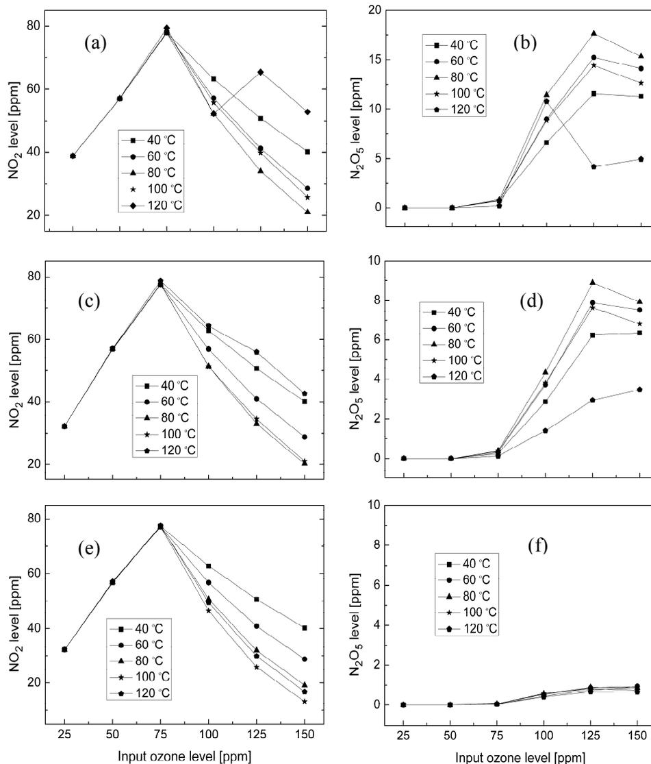
Fig. 9 Temperature dependent concentrations of  $NO_2$  (a), (c) and (e) and  $N_2O_5$  (b), (d) and (f) by calculations (a) and (b) without considering water sink effect for  $N_2O_5$ , (c) and (d) considering 100  $\mu m$  water droplets and (e) and (f) considering 10  $\mu m$  water droplets (residence time = 5 s,  $NO=80$  ppm).
