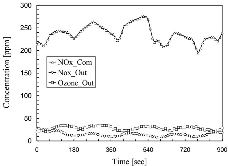
Fig. 18 NO<sub>x</sub> level commanding the ozone generator, NO<sub>x</sub>\_Com, and NO<sub>x</sub> and ozone levels after the scrubber, NO<sub>x</sub>\_Out and Ozone\_Out, respectively.
