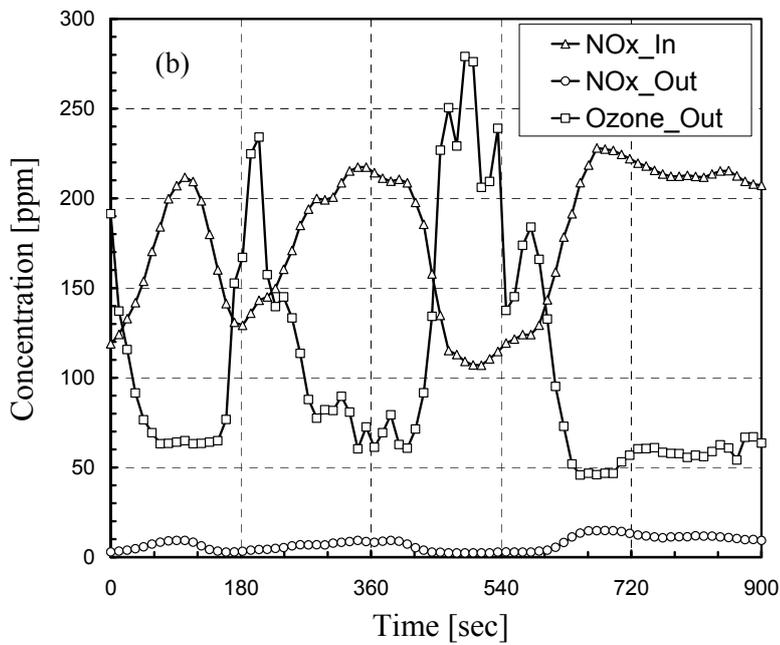
Fig. 14 NO<sub>x</sub> levels at the input and output of the reactor with the corresponding unconsumed ozone for a constant input of ozone of (a) 300 g/h and (b) 500 g/h.
