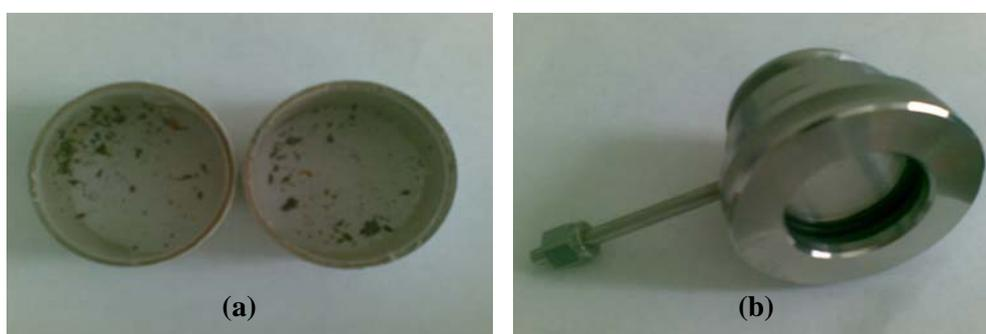
Fig 12 (a) Measurement windows contaminated with large dust particles; (b) Mounting system for observation window including a small pipe for pouring dry air.
