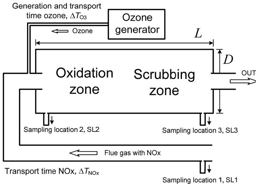
Fig. 16 Schematic of the optimization scheme.  $\text{NO}_x$  is sampled at locations SL1, SL2 and SL3 while ozone at SL2 and SL3.
