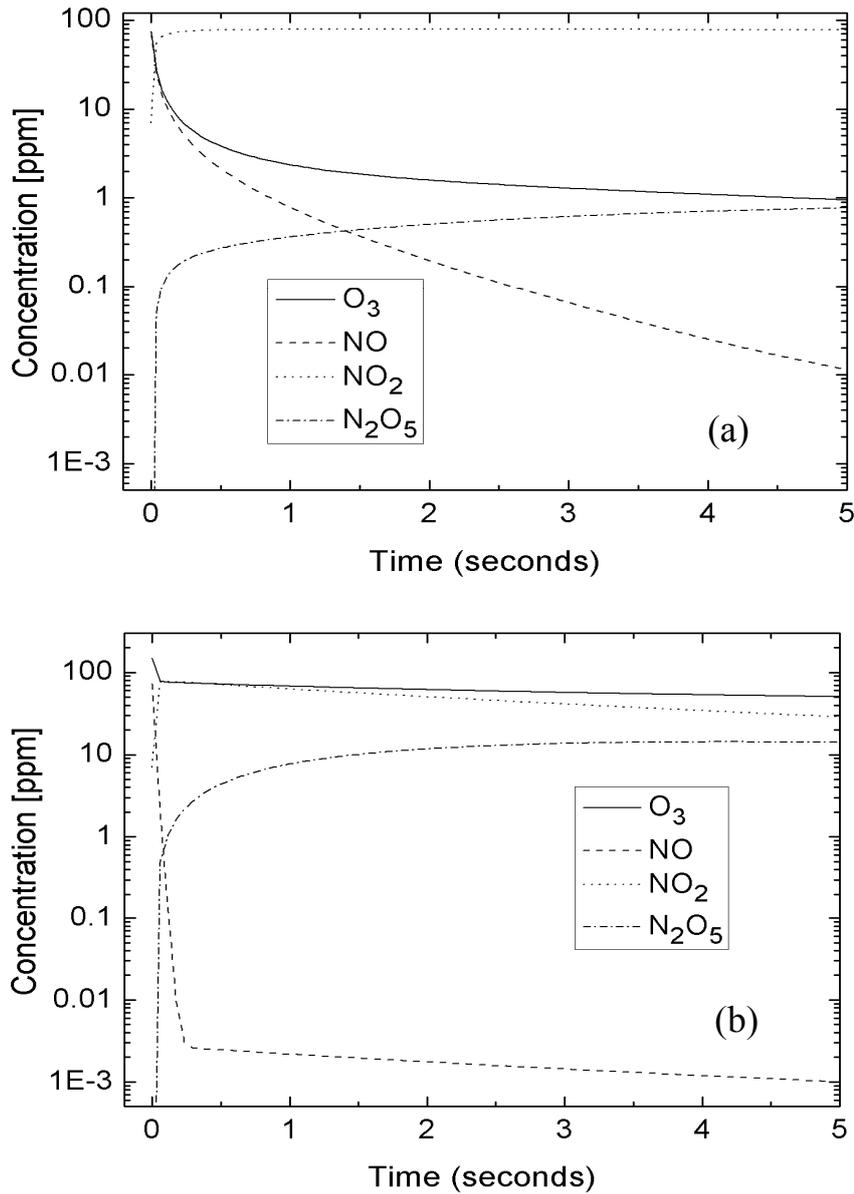
Fig. 3. Calculated evolutions of the concentrations of O<sub>3</sub>, NO, NO<sub>2</sub>, N<sub>2</sub>O<sub>5</sub> in the reactor during 5 seconds after ozone injection without considering any effects of heterophase reactions (a) 75 ppm ozone input, (b) 150 ppm ozone input.
