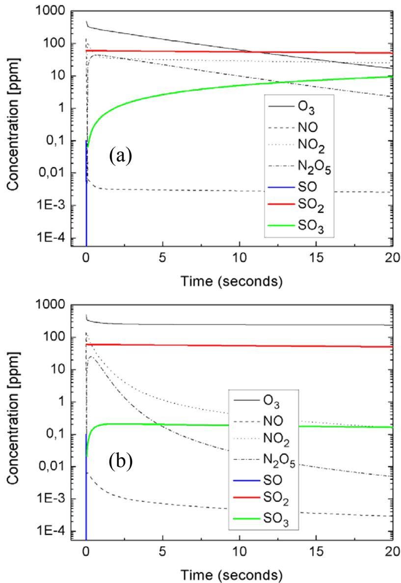
Fig. 11 Calculated evolutions of O<sub>3</sub>, NO, NO<sub>2</sub>, N<sub>2</sub>O<sub>5</sub>, SO, SO<sub>2</sub> and SO<sub>3</sub> concentrations in the reactor during 20 seconds after ozone and COI injection (100 ppm) (a) no water and (b) including 10 μm water droplets.
