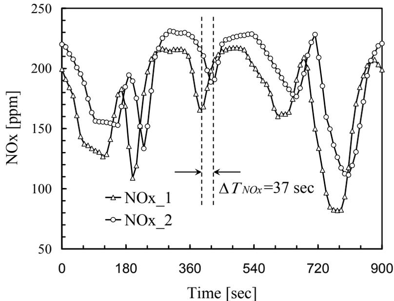
Fig. 17 NO<sub>x</sub> levels at two locations, 1 and 2, showing that a transportation line of 25 m between provides a time delay of 37 seconds. The 10 % difference in the NO<sub>x</sub> levels is attributed to different sensor calibration.
