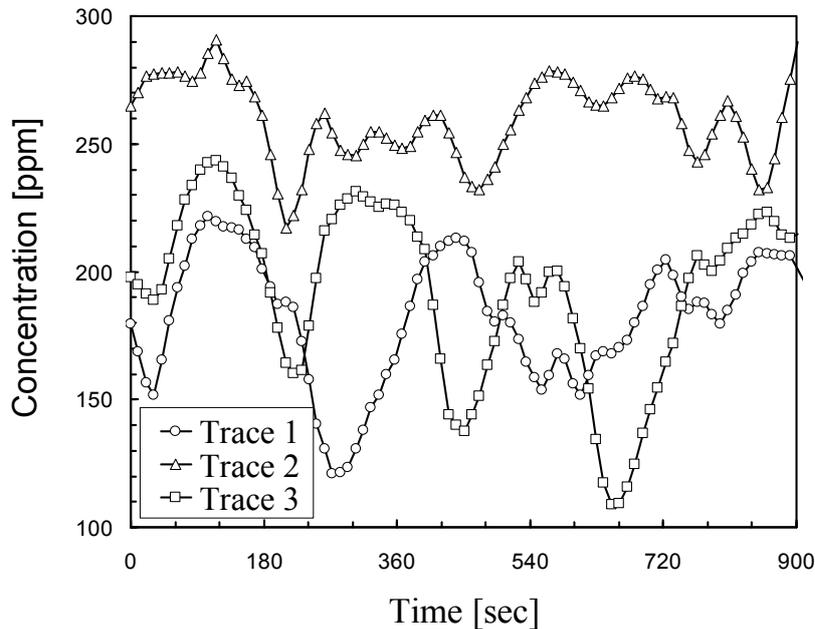
Fig. 13 Typical NO<sub>x</sub> levels as a function of time for a biomass power plant, showing very large variation within one minute time interval.
