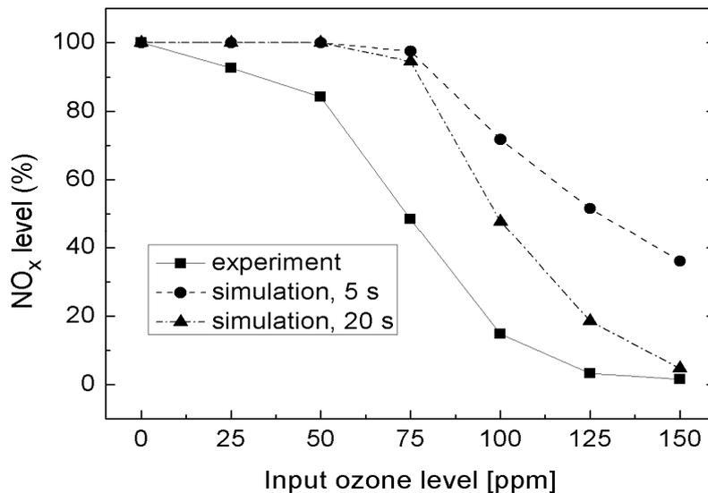
Fig.4 Remained NO<sub>x</sub> after the scrubber at different input ozone level by both experiment measurement and simulations for a residence time of 5 and 20 sec.
