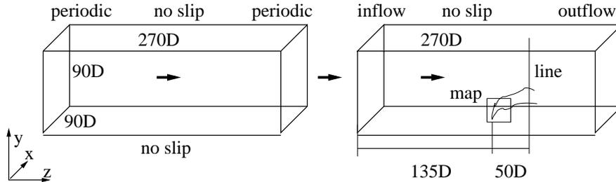
Figure 3: Geometry of the spray jet in crossflow
