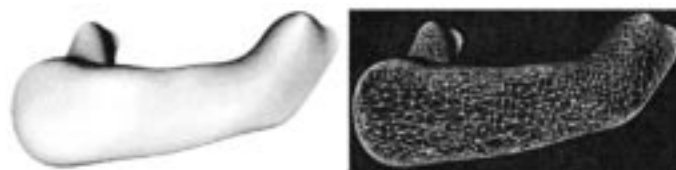
Fig. 8. Converged diffusion algorithm with a high value of \sigma_D ( \sigma_D = 10 mm). The surface and wire frame of the deformed surface are shown to the left and right, respectively. All folds remaining in the surface at the bottom of the previous figure are now gone.
