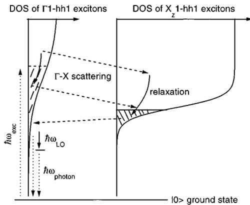
FIG. 2. Relaxation scheme of optically excited electron-hole pairs into ( $\Gamma1$ -hh1) local minima exciton states. From these states, the excitons decay radiatively, either with or without the emission of an GaAs LO phonon, as indicated by the dotted arrows. The relaxation involves the ( $X_z1$ -hh1) excitons as transport states. The localized states at the band edges of the densities of states (DOS) are hatched.
