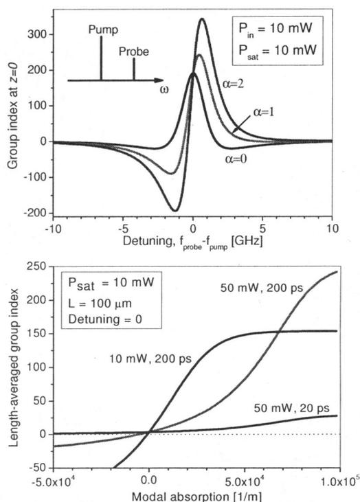
**Fig. 1.** Calculated variation of group index with detuning (top; at waveguide input for an absorption coefficient of  $5 \cdot 10^4 \text{ m}^{-1}$ ) and modal absorption (bottom; averaged over waveguide length).
