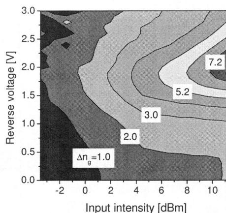
**Fig. 2.** Contour plot of measured change in group index versus input intensity and reverse voltage for a 100  $\mu\text{m}$  long semiconductor waveguide.
