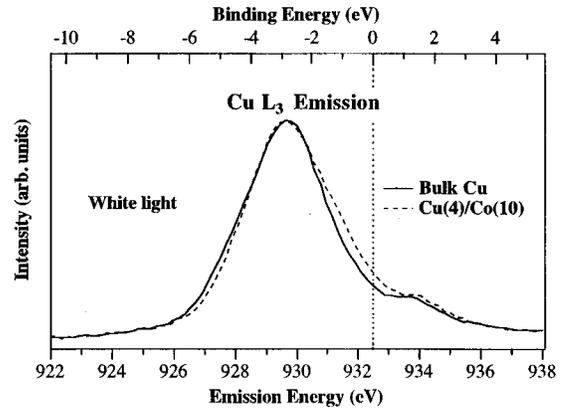
FIG. 5. Cu  $L_3$  XES spectra for bulk Cu (solid line) and Cu(4)/Co(10) (dashed line) excited with “white light,” i.e., broad bandpass x rays. Note sizable multielectron intensity above 932.4 eV, corresponding to the Fermi level position.
