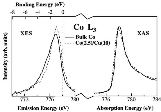
FIG. 2. Co  $L_3$  x-ray emission (XES) and absorption (XAS) spectra of a 200-Å Co film, denoted bulk Co, and the multilayer Si(100)/Ru(30 Å)/30×{Co(2.5 Å)/Cu(9.25 Å)}Ru(10 Å), denoted Co(2.5)/Cu(10). The energy scales of the spectra were determined as discussed in the text. The Co  $2p_{3/2}$  XPS binding energy relative to the Fermi level was taken to be 778.1 eV.
