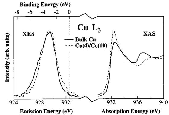
FIG. 3. Cu  $L_3$  x-ray emission (XE) and absorption (XA) spectra of a 200-Å Cu film, denoted bulk Cu, and the multilayer Si(100)/Ru(50 Å)/20×{Co(10 Å)/Cu(4 Å)}Ru(15 Å), denoted Cu(4)/Co(10). The energy scales of the spectra were determined as discussed in the text. The Cu  $2p_{3/2}$  XPS binding energy relative to the Fermi level was taken to be 932.4 eV.
