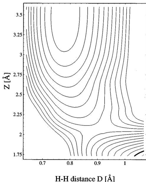
FIG. 3. Equipotential contours of the *ab initio* PES for  $D_2$  interacting with Si(100) at a fixed phonon coordinate of  $Y = 0$  Å. This produces contours about the symmetric transition state in terms of the center of mass distance of the  $D_2$  to the surface as measured by  $Z$  and the D–D distance  $D$ . The contour interval is 0.05 eV and the origin of energy is given as the surface at  $Y = 0$  (and  $Z$  large) plus the energy of a free  $D_2$ .
