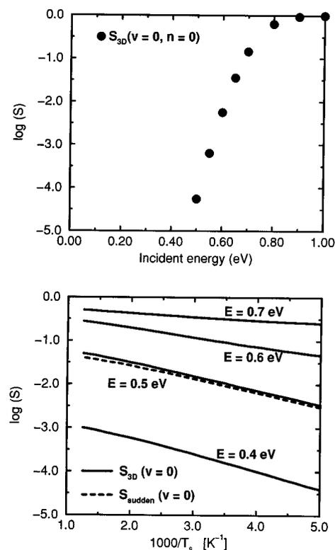
FIG. 9. Quantum dynamical calculations of the dissociative chemisorption probability  $S$  using the model PES  $U_{sym}$ .  $\log(S)$  is plotted as a function of initial energy for the ground  $D_2$  initial state and for  $T_s=0$  ( $n=0$ ) (top) and as a function of reciprocal surface temperature for different incident energies  $E$  (bottom). A sudden calculation of  $S$  at  $E=0.5$  eV is also given for comparison in the bottom part of the figure.
