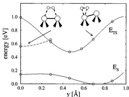
FIG. 1. Total energy of the asymmetric and symmetric transition states  $E_{TS}$  for  $D_2$  interacting with Si(100) and of the clean surface  $E_s$  as a function of the Si dimer phonon coordinate  $Y$ .
