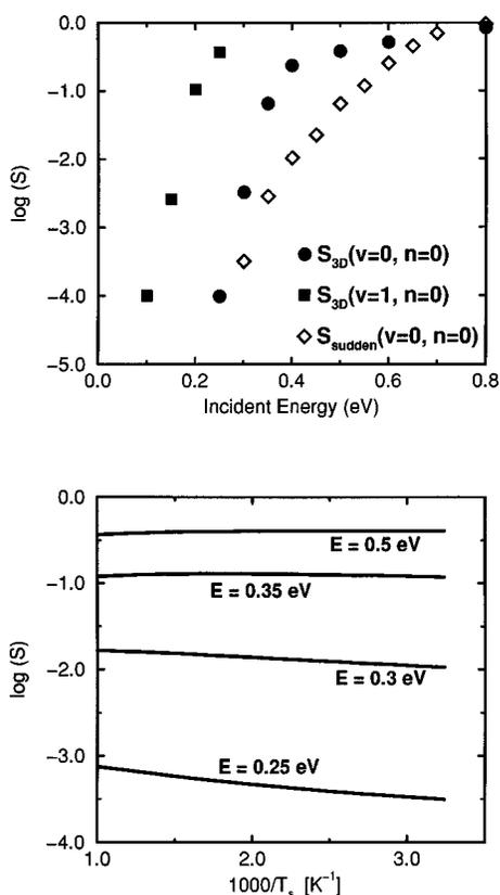
FIG. 8. Quantum dynamical calculation of the dissociative chemisorption probability  $S$  using  $U_{\text{asym}}$  as the PES  $\log(S)$  is plotted as a function of initial energy for different initial  $\text{D}_2$  vibrational states  $v$  and for  $T_s=0$  ( $n=0$ ) (top) and as a function of reciprocal surface temperature for different incident energies  $E$  (bottom). A sudden calculation of  $S$  is also given for comparison in the top part of the figure.
