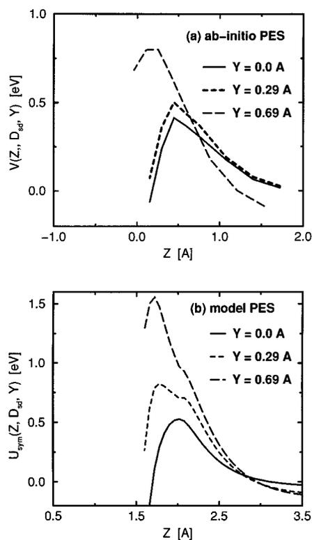
FIG. 7. Comparison of the model  $U_{\text{sym}}$  to the *ab initio* “bare” PES in the general region of the symmetric transition state. Several one-dimensional “cuts” through the PES are presented at different  $Y$ . The potential energy  $V(Z, D_{\text{sd}}, Y)$  is plotted against  $Z$ .  $D_{\text{sd}}$  is the value of  $D$  obtained at each  $Z$  by steepest descent on the PES at a fixed  $Y=0$ . (a) *ab initio* PES and (b) model  $U_{\text{sym}}$ .
