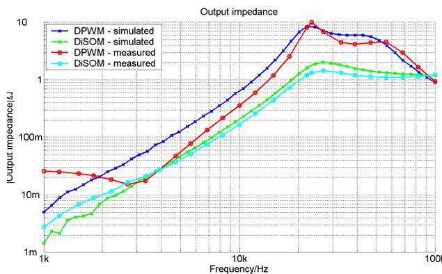
Fig. 13: Simulated and measured output impedance versus frequency
