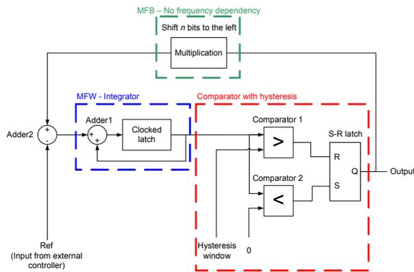
Fig. 3: Block diagram of the DiSOM modulator
