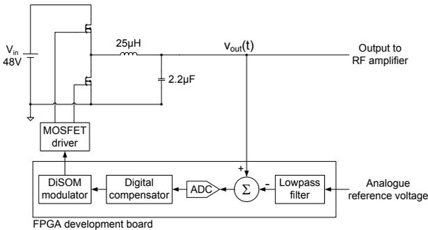
Fig. 6: Block diagram for the DiSOM based design
