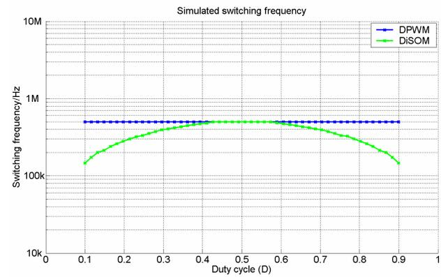
Fig. 9: Simulated switching frequency versus duty cycle
