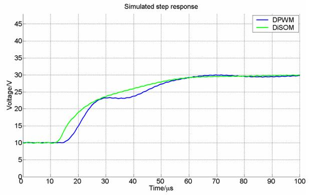
Fig. 14: Simulated step response
