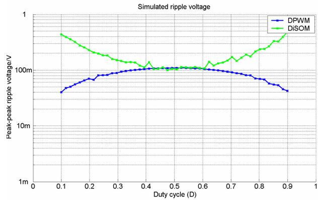
Fig. 8: Simulated ripple voltage versus duty cycle
