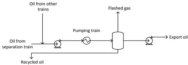
Figure 3: Flow sheet of the export pumping section
