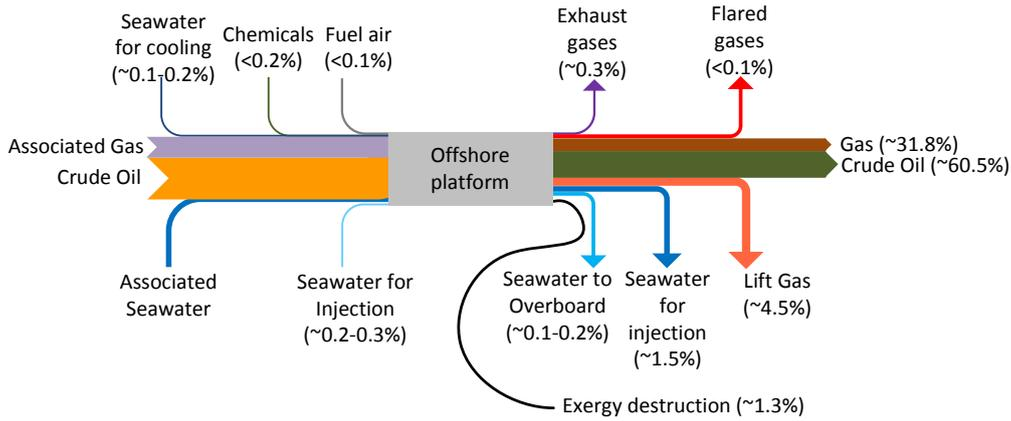
Figure 8: Grassmann diagram of the offshore oil and gas platform – Baseline Case
