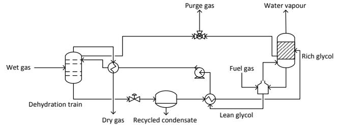
Figure 4: Flow sheet of the dehydration train
