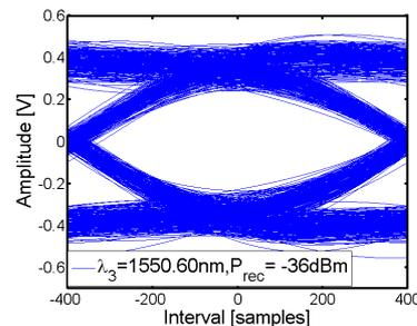
Figure 5. Eye diagram of the demodulated WDM channel
