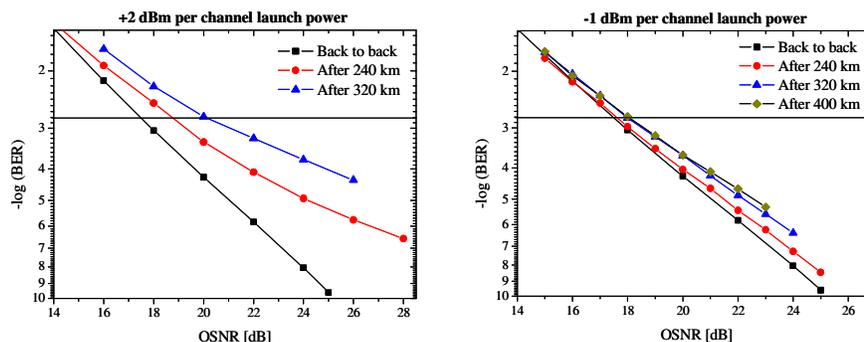
Fig. 3: Measured BER of one 32.1 Gbit/s RZ-D8PSK channel in a WDM system with 24 NRZ channels. Launch power +2 dBm per channel (left) and -1 dBm per channel (right)
