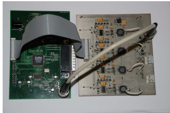
Figure 5. Prototype converter (right) and FPGA board (left)
