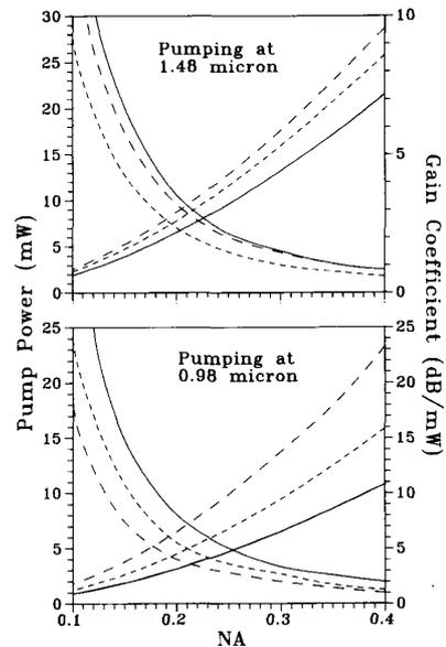
Fig. 3. Input pump power (decreasing curves) and gain coefficient versus NA in step index  $\text{Er}^{3+}$  fibers. Upper figure: pumping at 1.48  $\mu\text{m}$ . Lower figure: pumping at 0.98  $\mu\text{m}$ . Solid curves: the index raising co-dopant is aluminum. Small dashes: the index raising co-dopants are aluminum and germanium. Long dashes: the index raising co-dopant is germanium.
