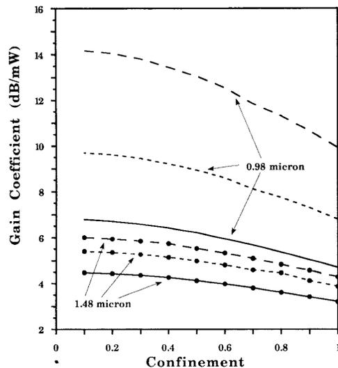
Fig. 4. Gain coefficient versus erbium confinement in step index  $\text{Er}^{3+}$  fibers with an NA of 0.25. Marks: pumping at 1.48  $\mu\text{m}$ . No marks: pumping at 0.98  $\mu\text{m}$ . Solid curves: the index raising co-dopant is aluminum. Small dashes: the index raising co-dopants are aluminum and germanium. Long dashes: the index raising co-dopant is germanium.
