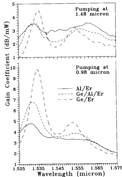
Fig. 5. Gain coefficient versus signal wavelength in step index  $\text{Er}^{3+}$  fibers with an NA of 0.25. Upper figure: pumping at 1.48  $\mu\text{m}$ . Lower figure: pumping at 0.98  $\mu\text{m}$ . Solid curves: the index raising co-dopant is aluminum. Small dashes: the index raising co-dopants are aluminum and germanium. Long dashes: the index raising co-dopant is germanium.
