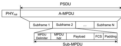
Fig. 1. Frame structure in A-MPDU packet aggregation scheme
