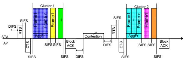
Fig. 2. Contention and transmission procedure in *one4all* scheme
