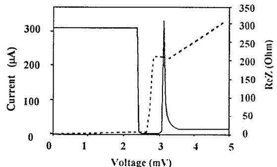
FIG. 1. Real part of the microwave impedance,  $\text{Re } Z$ , of the SIS junction as function of the bias voltage,  $V$ , calculated at frequency  $f = eV_g/10h = 70 \text{ GHz}$ . The model IVC, with normal state resistance  $R_n = 15 \Omega$ , used in the simulation is shown by the dashed line.
