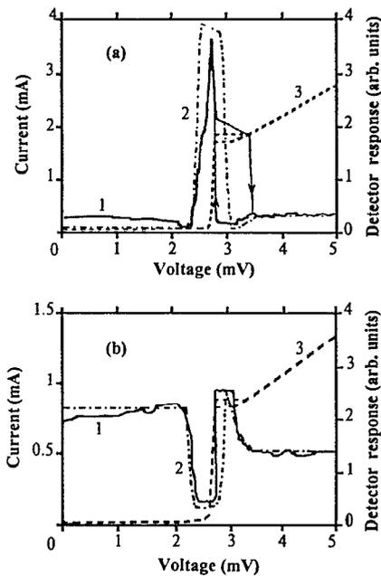
FIG. 4. Experimental (1) and simulated (2) detector response vs bias voltage of the series (a) and parallel (b) attenuators. Model *IVC*'s of the corresponding attenuators are shown by the dashed curve (3).
