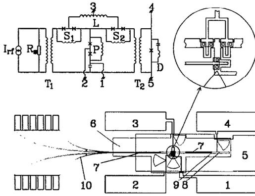
FIG. 2. Equivalent diagram and layout of the integrated attenuator circuit. 1–5—contact pads; 6—SiO<sub>2</sub> isolation; 7—microwave quarter-wave transformers, 8—tuning-out microstrip stub; 9—SIS detector; 10—fin-line antenna.
