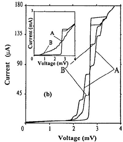
FIG. 3.  $IVC$ 's of the SIS detector at different bias voltages at input frequency  $f = 74.6 \text{ GHz}$  showing action of the series attenuator (S-att) at low level (top) and high level (bottom) of the input power. Insert shows the corresponding  $IVC$ 's of the S-att.
