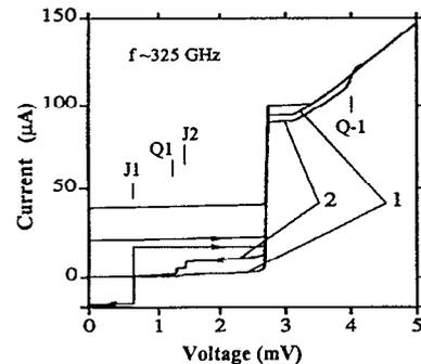
FIG. 5. *IVC* of a SIS detector at two levels of applied power from an on-chip integrated flux-flow oscillator (FFO,  $f=325$  GHz). The power was adjusted by a superconducting attenuator inserted in the line between the FFO and the detector. Symbols  $J_N$  and  $Q_N$  refer to the  $N$ 'th rf-induced Josephson step and quasiparticle step, respectively.
