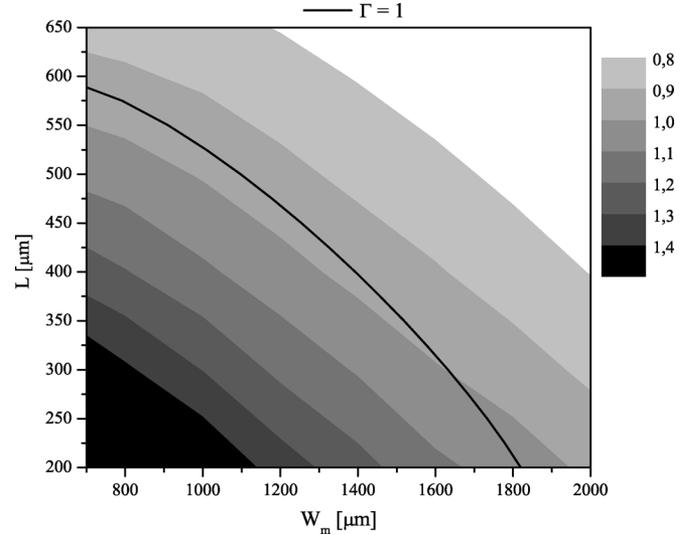
Fig. 8. The ratio between the mean strains,  $\overline{\epsilon_{x_h}}/\overline{\epsilon_{x_v}}$ , plotted in Figs. 6 and 7, respectively, is shown in this figure. The filled contour plot is the FEM model and the black line is based on the analytical model. The relative sensitivity is equal to one along the black line according to the analytical model and again there is good agreement with the FEM model.
