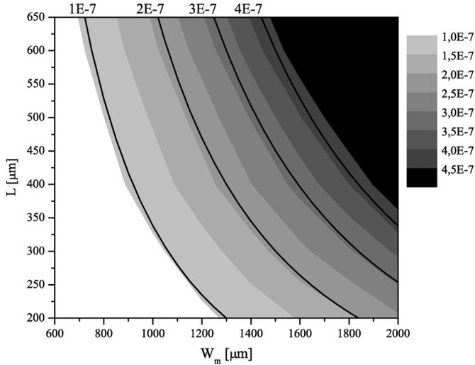
Fig. 6. The mean strain,  $\overline{\epsilon_{x_v}}$ , for accelerations in the vertical direction as a function of seismic mass width  $W_m$ , and beam length  $L$ . The filled contour plot are the FEM model results, while the black lines are the analytical model results. Increasing beam length and increasing mass width increases the mean strain.
