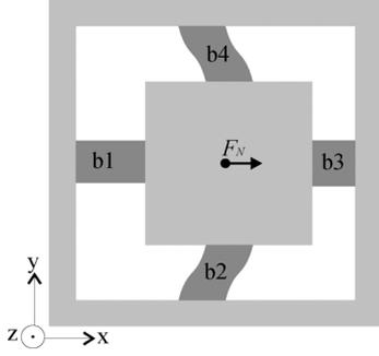
Fig. 5. Top view of the seismic mass and the four beams deflected due to an horizontal acceleration. This movement results in a lateral force  $F_N$ . The beams  $b_2$  and  $b_4$  are bending, beam  $b_1$  is stretched, and beam  $b_3$  is compressed.
