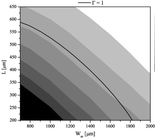
Fig. 12. The ratio,  $\overline{\sigma_{T_h}}/\overline{\sigma_{T_v}}$ , between the total mean stresses for vertical and horizontal accelerations. The full line is the contour  $\overline{\sigma_{T_h}}/\overline{\sigma_{T_v}} = 1$  according to the analytical model. As in Fig. 8, there is a very good agreement between the analytical model and the FEM model.
