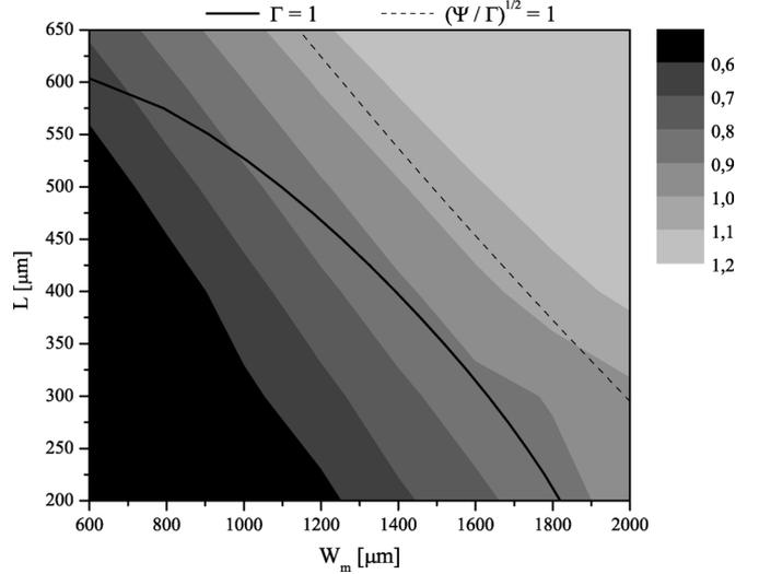
Fig. 13. The contours show the ratio  $\omega_h/\omega_v$ , between the horizontal resonant frequency and the vertical resonant frequency calculated using the FEM model. The contour of relative sensitivity equal to one (full line) is shown for comparison. The dashed line is the contour  $\sqrt{\Psi/\Gamma}$ .
