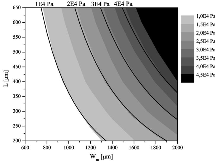
Fig. 10. The total mean stress,  $\overline{\sigma_{T_v}}$ , in the PZT on the beam for vertical accelerations. The full lines are results from the analytical model. The agreement is seen to be excellent.
