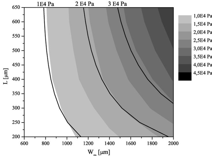
Fig. 11. The total mean stress,  $\overline{\sigma_{T_h}}$ , in the PZT on the beam for horizontal accelerations. The full lines are results from the analytical model. Good agreement between the FEM model and the analytical model is seen, for longer beams the agreement becomes less good.
