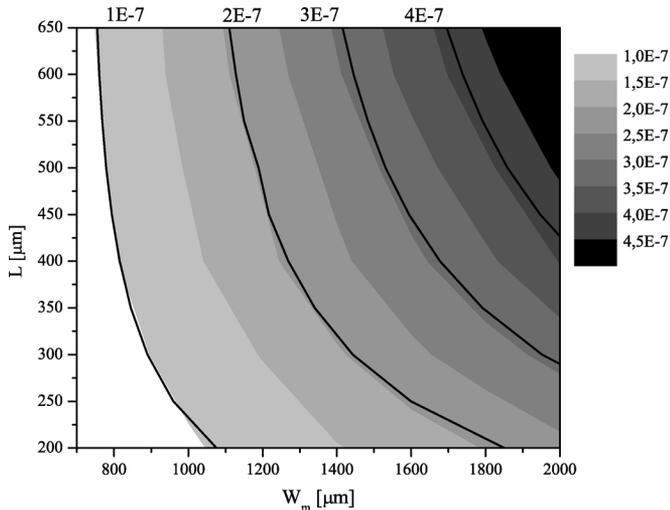
Fig. 7. The mean strain,  $\overline{\epsilon_{x_h}}$ , for horizontal accelerations as a function of mass width  $W_m$ , and beam length  $L$ . The filled contour plot are the FEM model results, while the full lines are the analytical model results. Increasing beam length and increasing mass width increases the mean strain.
