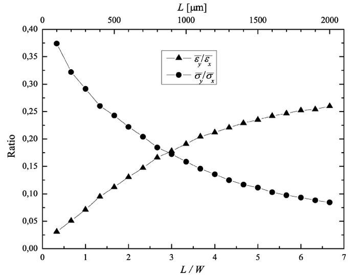
Fig. 9. The ratios  $\overline{\epsilon_y}/\overline{\epsilon_x}$  and  $\overline{\sigma_y}/\overline{\sigma_x}$  as a function of the beam length-width ratio,  $L/W$ , calculated using the FEM model ( $W = 300 \mu\text{m}$  is fixed and  $L$  is varied from  $100 \mu\text{m}$  to  $2000 \mu\text{m}$ , the other parameters are shown in Table II).
