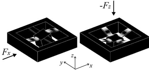
Fig. 3. The figure shows the two modes of operation, a horizontal acceleration (left) and a vertical acceleration (right). The grayscale indicates the strain energy density, [ $\text{Jm}^{-3}$ ], in arbitrary units where the bright gray represents a large value.
