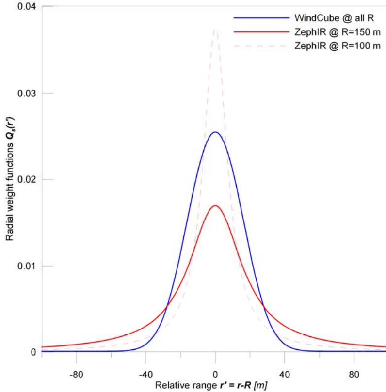
**Fig. 2:** The cw ZephIR and the pulsed WindCubes sounding volumes radial wind speed resolution functions intercompared at fixed measurement range  $R=150$  m. The stippled curve represent the ZephIR's radial sounding volumes resolution at range  $R = 100$  m.
