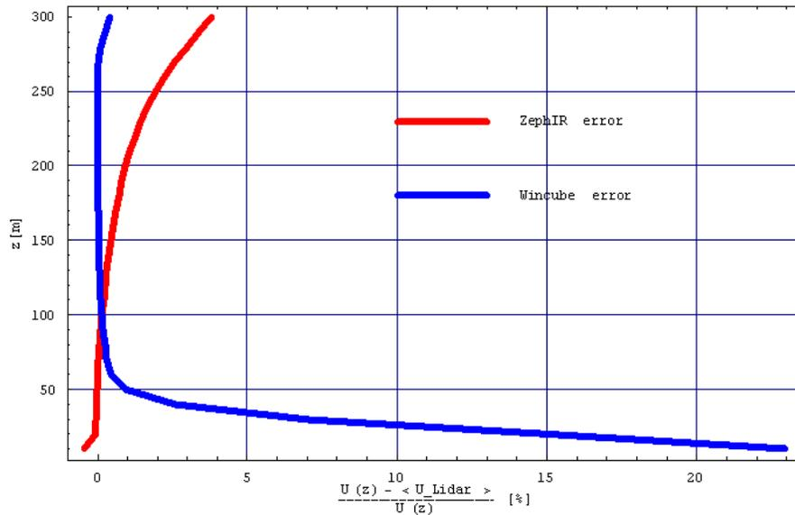
Fig.3: Prediction of the relative sounding volume induced relative errors on lidar-measured neutral mean wind profiles, as function of range  $z$ . The corresponding relative wind speed measurement error as function of height using a 30 degree wedge can be obtained by multiplying the ordinate with  $\sqrt{3}/2 \sim 0.87$ .
