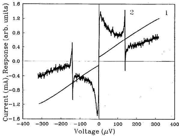
FIG. 1. The  $IV$  characteristic (1) and the response  $\Delta V(V)$  (2) to 70.2 GHz radiation for a  $\text{YBa}_2\text{Cu}_3\text{O}_7$  SEJ32 at 77.3 K.
