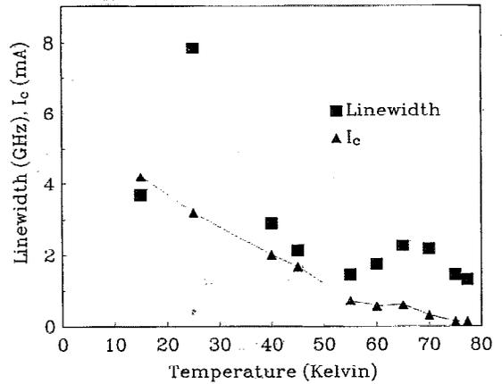
FIG. 3. The linewidth of 70.2 GHz Josephson radiation (squares) and critical current ( $I_c$ ) (triangles) of  $\text{YBa}_2\text{Cu}_3\text{O}_7$  SEJ32 as function of temperature. The solid line is a guide to the eye.
