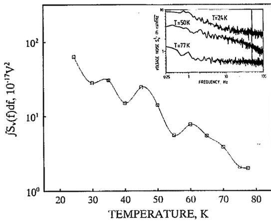
FIG. 4. The integral voltage noise in a bandwidth from 0.25 Hz to 3 kHz vs temperature for SEJ32 at bias voltage  $145 \mu V$ . The insert shows the spectral density of the voltage fluctuations at  $V=145 \mu V$  for different temperatures.
