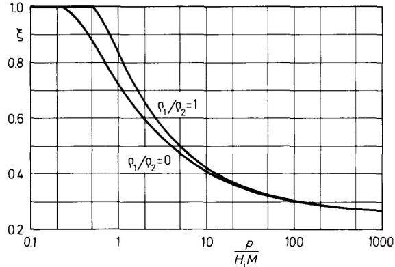
Figure 2. Influence of electrode microscopic curvature  $H_i$  upon the surface roughness factor  $\xi$ .
