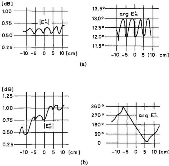
Fig. 4. Examples of recorded curves. (a) Movement of test object. (b) Movement of receiving horn.
