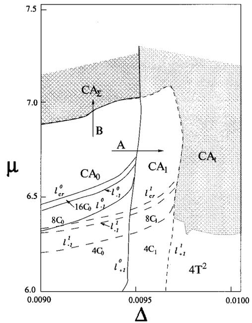
FIG. 1. Bifurcation diagram for two coupled Rössler systems ( $\alpha=0.15$ ,  $\beta=0.2$ ,  $c=0.02$ ). The solid curves are bifurcation lines of ‘‘in-phase’’ attractors. The dashed curves show bifurcations of ‘‘out-of-phase’’ attractors.
