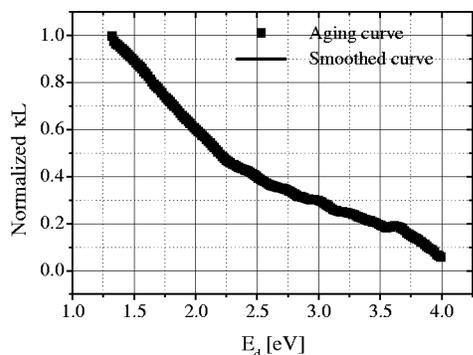
FIG. 15. Aging curve obtained from an average of the 0.25 and 0.0025 K/s decays when the demarcation energy is calculated for frequency  $\nu = 10^{14.5} \text{ s}^{-1}$ . The curve is not as smooth as that for the grating written in the unloaded fibered. We believe that this is due to interference but do not know the origin.
