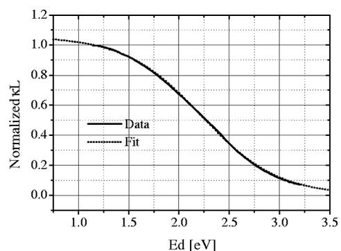
FIG. 9. Final aging curve found from the average of 0.25 and 0.0036 K/s. A fit of the aging curve to Eq. (8) gave the parameters  $A = 1.06$ ,  $E_{\text{center}} = 2.2 \text{ eV}$ , and  $\Delta = 0.38 \text{ eV}$ . The two curves overlap well.
