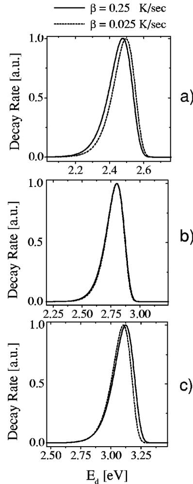
FIG. 1. Theoretical rate of decay for 2.8 eV activation energy and an attempt frequency  $\nu = 10^{13} \text{ s}^{-1}$ . The decay rate at two values of  $\beta$  is plotted against the demarcation energy,  $E_d$ , for different trial attempt frequencies,  $\nu_t =$  (a)  $10^{11}$ , (b)  $10^{13}$ , and (c)  $10^{15} \text{ s}^{-1}$ . It is seen that when the trial frequency is correct the curves overlap and are peaked at the correct energy.
