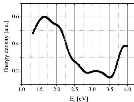
FIG. 16. Energy distribution of defects for gratings written in  $D_2$  loaded fiber obtained by differentiating the smoothed curve. It can be seen that there are two different distributions, indicating two defect types.
