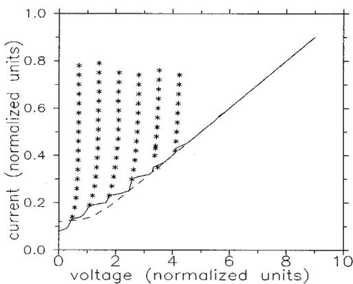
FIG. 2. The  $I-V$  curves with uniform bias (dashed line) and the nonuniform (solid line) for a two-junction stack obtained by decreasing the bias current. We also show the full height of the ZFS, obtained increasing the bias to nonuniform profile, with marks. In this figure,  $L=10$ ,  $\alpha=0.1$ , and  $\epsilon=0.3$ .
