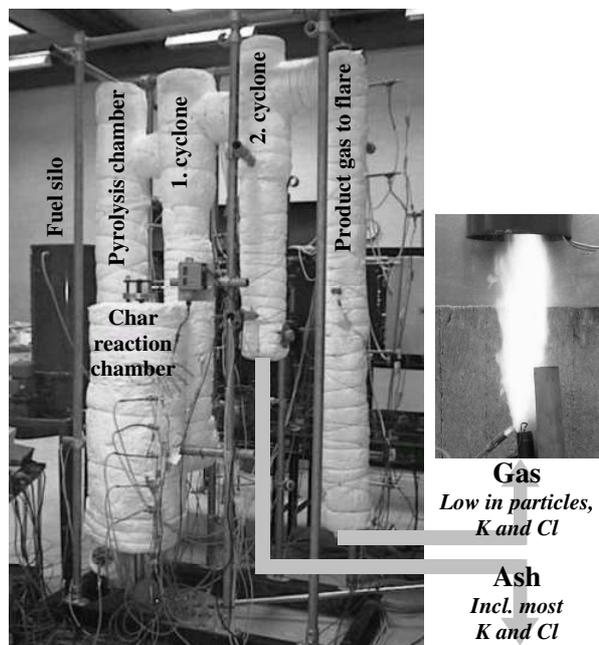
Figure 1: Picture of 50 kW LT-CFB test plant and flare burning product gas
