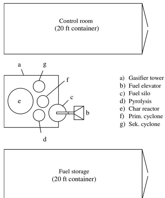
Figure 6: 500 kW LT-CFB plant at DTU, plan view.
