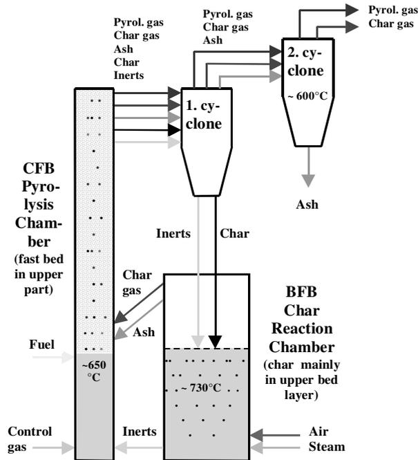
Figure 2: Flow diagram of LT-CFB concept
