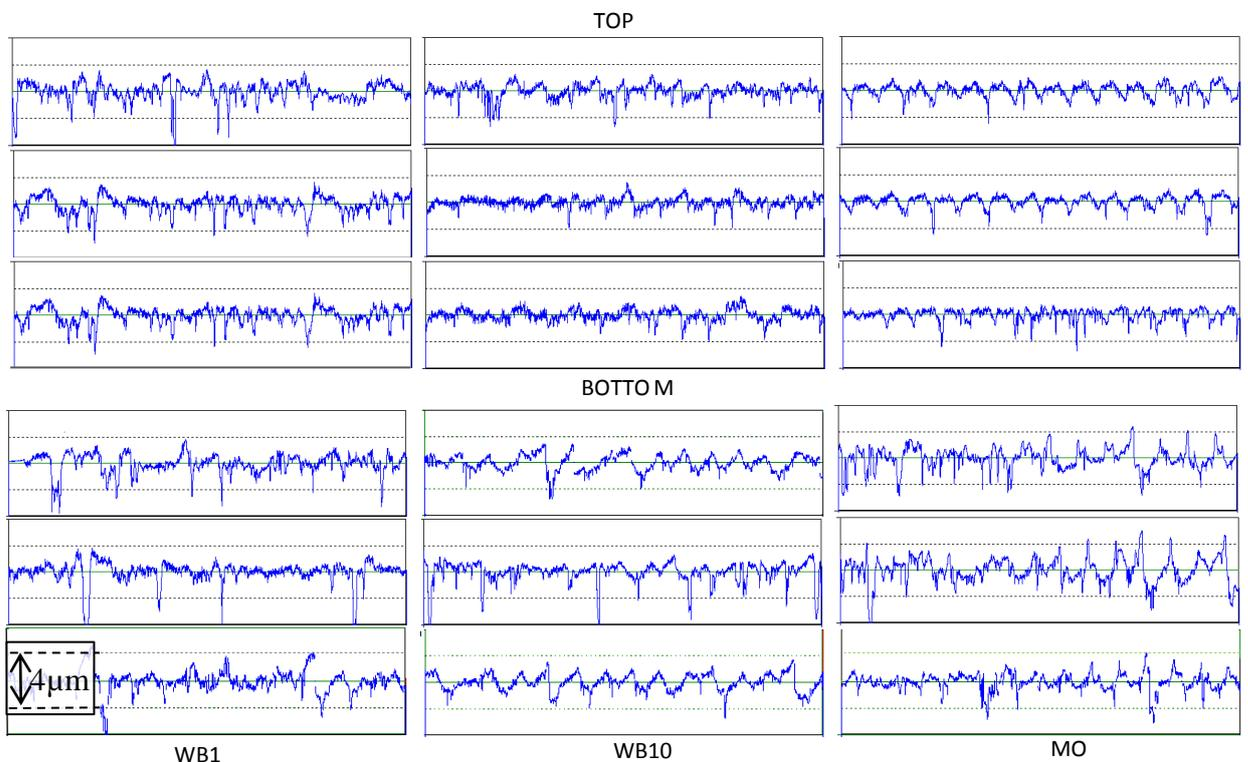
**Fig. 4: Nature and reproducibility of surface roughness profiles of reamed holes with different cutting fluids: WB1 (left), WB10 (middle) and MO (right). Length of all the profiles is 4 mm, vertical scale is shown in the left bottom figure.**
