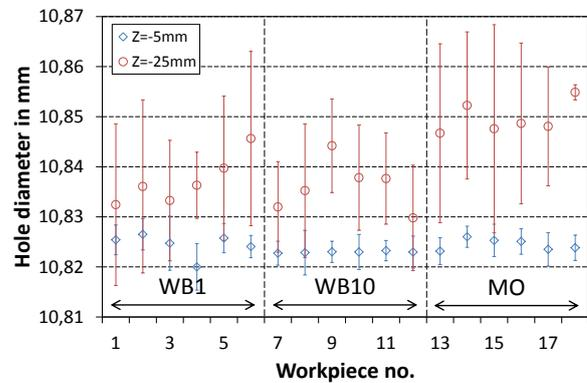
**Fig. 6: Reproducibility of the reamed hole diameter measured at two different levels along specimen height (top Z=-5 mm and bottom Z=-25 mm) for the three tested cutting fluids. Error bars represent the experimental standard deviation from three operators.**
