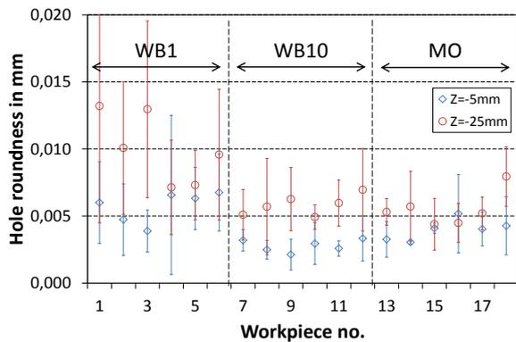
**Fig. 8: Reproducibility of the reamed hole roundness measured at two different levels along specimen height (top Z=-5 mm and bottom Z=-25 mm) for the three tested cutting fluids. Error bars represent the experimental standard deviation from three operators.**
