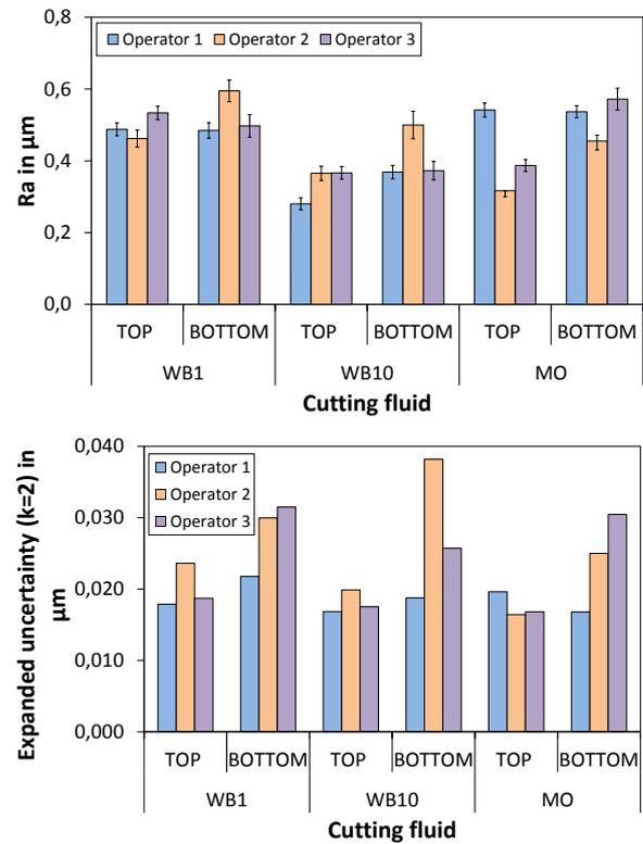
**Fig. 3: Results of the average surface roughness parameter Ra (top), measured by three operators at the top and at the bottom of reamed holes for each tested cutting fluid, and associated expanded uncertainties (bottom).**
