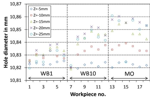
**Fig. 5: Reamed hole diameter measured at five different levels along specimen height for the three tested cutting fluids.**
