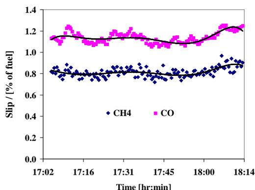
**Figure 2** The percentage of the fuel components CO and CH<sub>4</sub> that passes unburned through the engine,  $\lambda=1.4$ .
